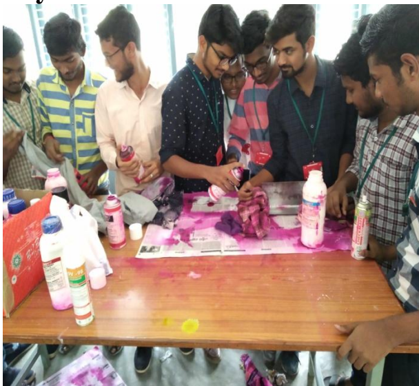
Hands On Experience By Students Conducting And Identifying Defects on Non Ferrous Materials By Liquid Penetrate Testing.
